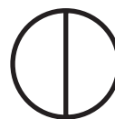
FIGURE A.17.3(c) Symbol that Represents Alternatively Act as Start and Stop or On and Off — IEC Symbol Number 5010.
