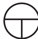
FIGURE A.17.3(d) Symbol that Represents Movement When Pressed and Stop Movement When Released (Jogging) — IEC Symbol Number 5011.
